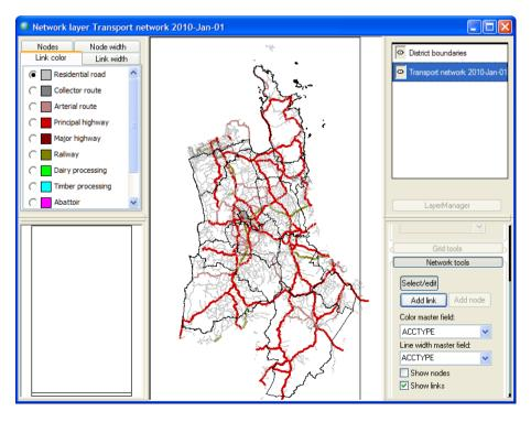
The figure below shows the network map window opened via the modeller user interface. Only the expansion roads added for 2010 are displayed.
